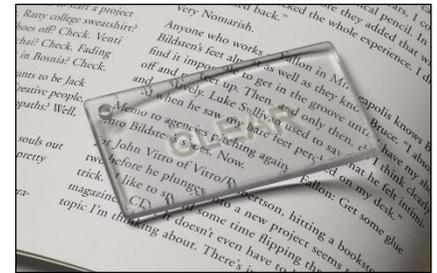
Figure 1: Polished and lacquered part, printed with VeroClear
